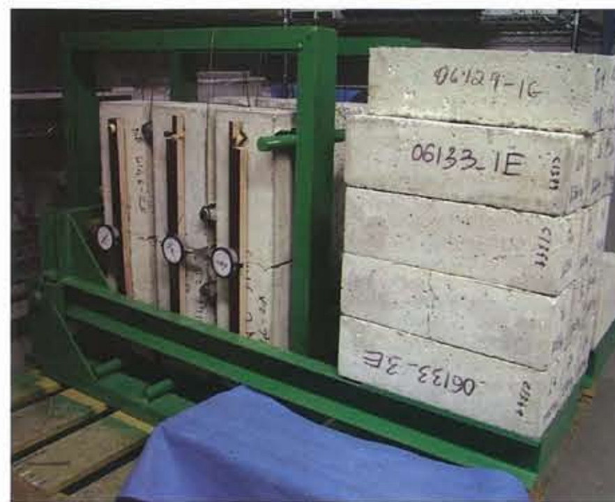
Figure 5: Loading frame to measure creep of cracked-fibre-reinforced concrete beams.
