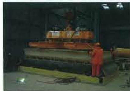
Figure 2: Revetment unit being vacuum-lifted out of the mould.
